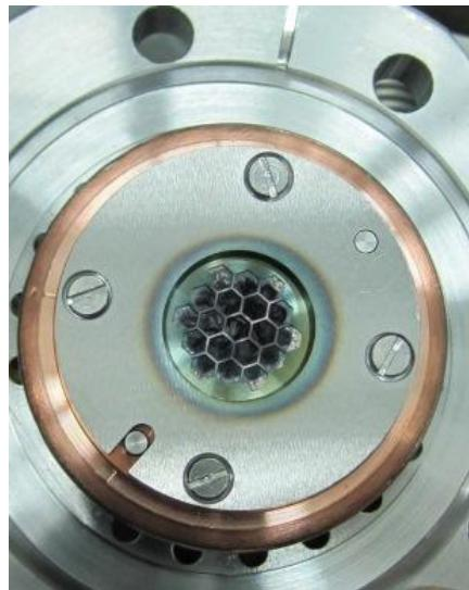
View of the immovable target placed between two honeycomb water cooling holder 85% transparency
