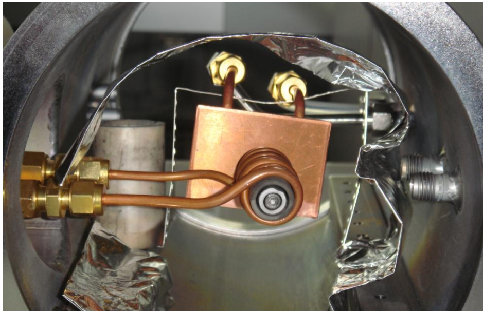
(1) Metal matrix, (2) Ta-crucible, (3) Corundum space holder, (4) Copper coil for induction, (5) Cooling for the furnace, (6) Vacuum window, (7) Cooled carrier holding, (8) Foil to collect released products
