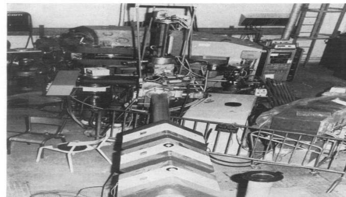
Electrostatic separator + Double Focusing spectro- Magnetic analyser
