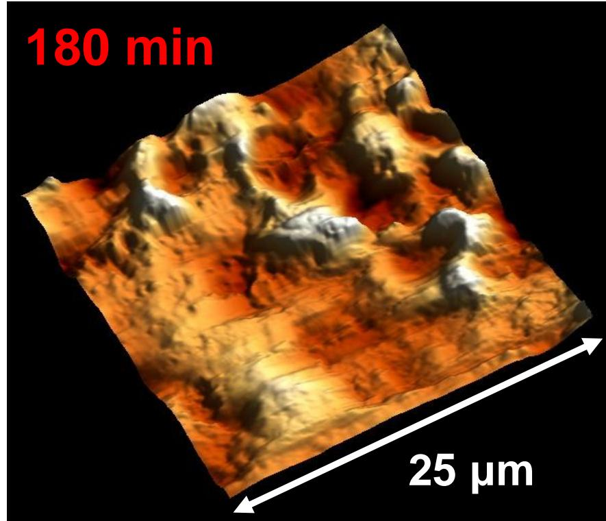
Deposition starts at spots (defects) on Ti-foil surface. Layer growth and **final layer stability** strongly depends on original backing surface roughness. Basic studies on layer formation and layer growth using AFM in solution. [A. Vascon et al., Nucl. Instr. and Meth. A, in press]
