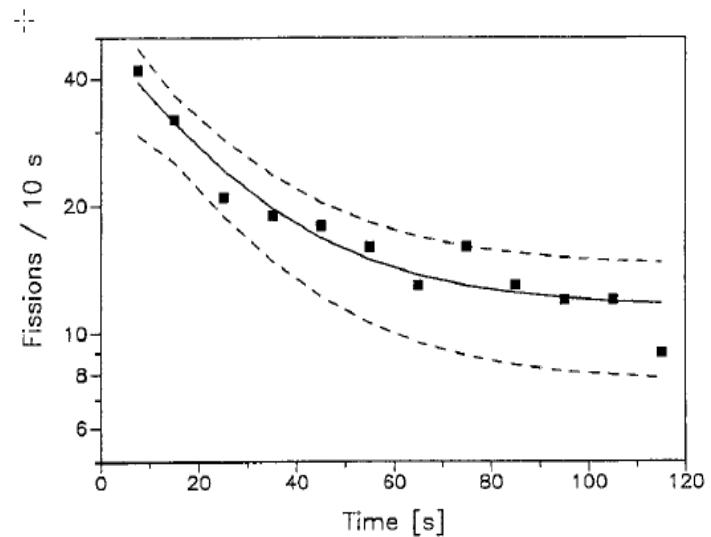
Fig. 2. Spontaneous fission activity measured in the  $^{18}\text{O} + ^{249}\text{Bk}$  reaction during a direct catch experiment with a beam dose of  $8.7 \cdot 10^{16}$  particles. The fit to the data results in a short-lived component with  $T_{1/2}=28 \pm 8$  s and a long-lived component from  $^{256}\text{Fm}$ , produced in this reaction via ingrowth from  $^{256}\text{Md}$
