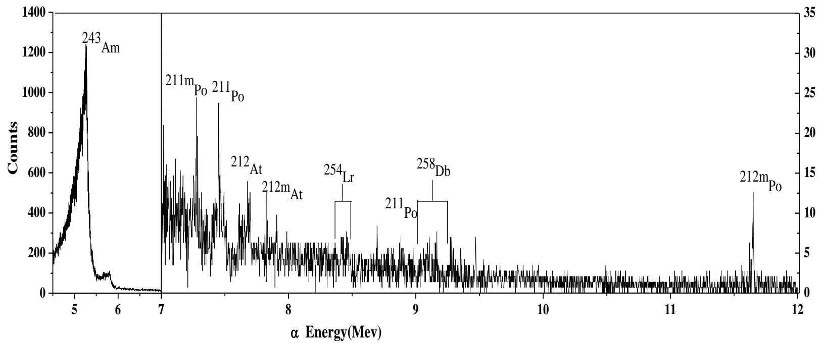
**Figure.** The sum  $\alpha$  -spectrum of detector 1 at isothermal temperature of 200 °C and 150 °C for 63 hours
